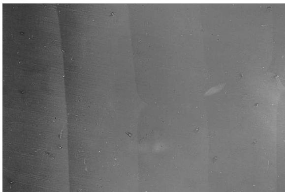
Figure 3. Photomicrograph of the Grandjean-Cano lines formed in the N^* phase of compound 11 at 134^\circ\text{C} .
